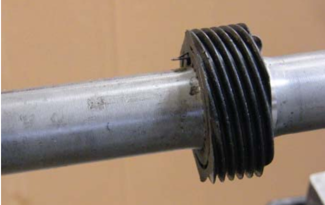
Figure 12. Here the gear is fully installed and tapped slightly to the rear to allow the tang to "bite" into the side of the plastic gear. Make sure that the clip is straight and square in the slot on this gear.
