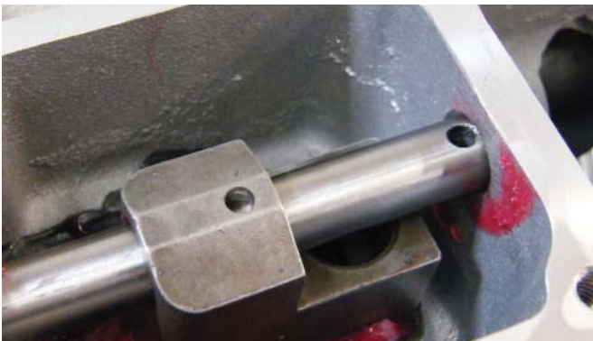
Figure 17. Here's a shot of the shift shaft entering the hole between the walls
