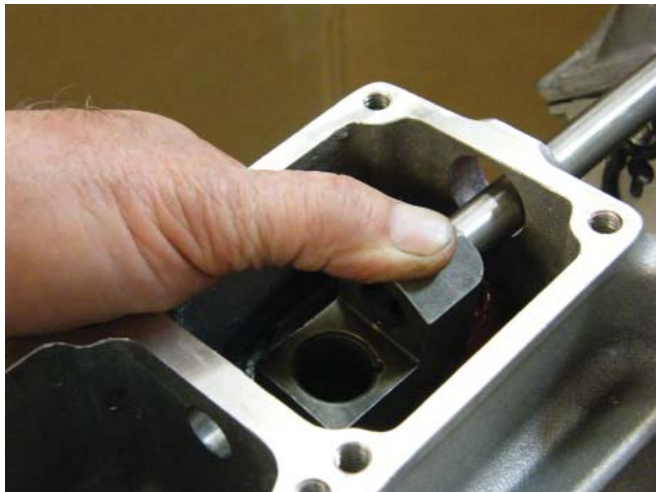
Figure 16. Again holding the shift block with your thumb, you guide the tailhousing assembly over the output shaft and the shift shaft. You will guide this assembly allowing the shift shaft to pass through the shift block toward the hole between the shift boxes seen at the bottom of this picture.
