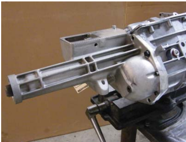
Figure 1. Here's the trans, mounted in the vise, ready for dis-assembly
