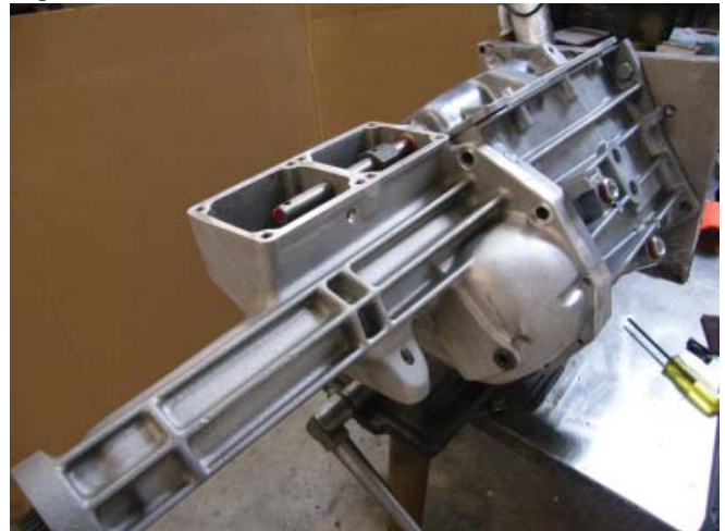
Figure 4. Here's the tailhousing, ready to be removed from the main case. I hope you've drained all the oil out of the transmission by this point, or you will be getting a major flood as you tap the tailhousing to the rear. In this shot, you can see the main case bolted to a plate held in the jaws of the vise to support the assembly.
