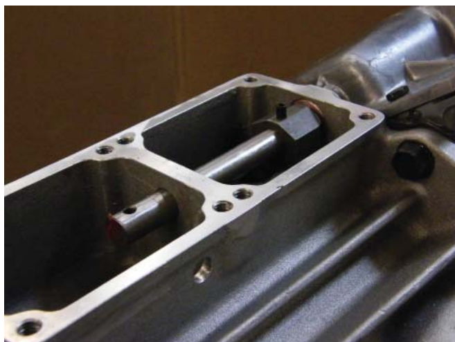
Figure 19. Drive the split pins in until they are flush with the top of the blocks
