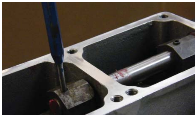
Figure 2. Use a 3/16 drift pin to tap the split pins down into the bodies of the shift blocks. You should be able to remove the rear block from the shift box at this point. Then continue driving the pin out the bottom. Note this block has no tang on the bottom
