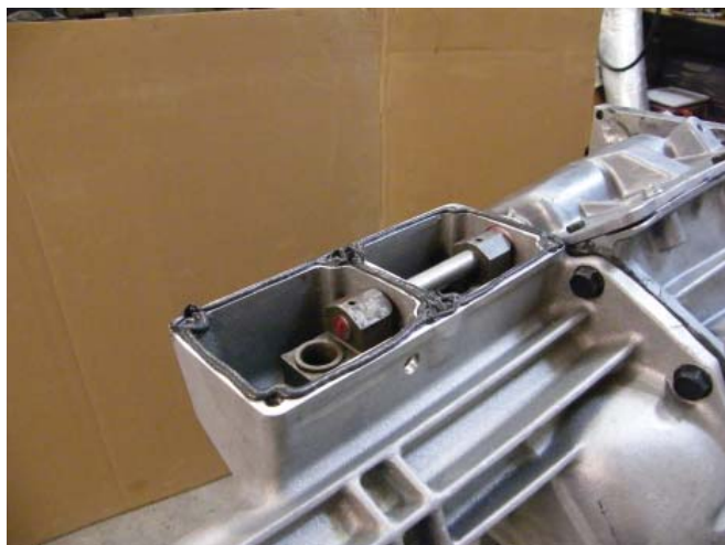
Figure 20. With the split pins in place, it's time to install the cover plate over the shift boxes with all six bolts. I typically wait a day for the RTV to set on this cover plate before I remove four bolts and the shifter for installation in the Tiger. Then some grease on the ball end of the shift lever and more RTV on the perimeter of the shift mechanism before it's lowered into place through the tunnel floor. I hope this makes the assembly clear and easier for you.
