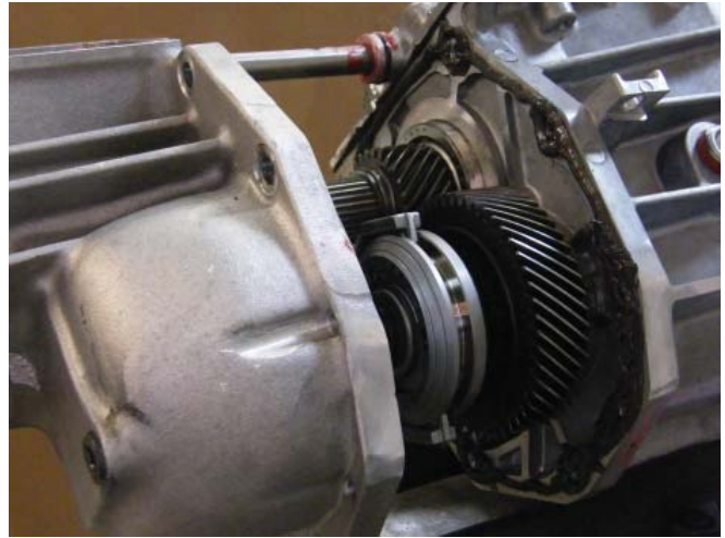
Figure 13. Here's a shot showing the RTV sealant placed on the main case. You can see the loops around the bolt holes and the extra sealing material in the 1/4" bolt area. I only apply the RTV to one side of the assembly. Note that the rear bearing race is about where you want it to be. It sticks out of the main casting the same distance as the bearing recess in the tailhousing.
