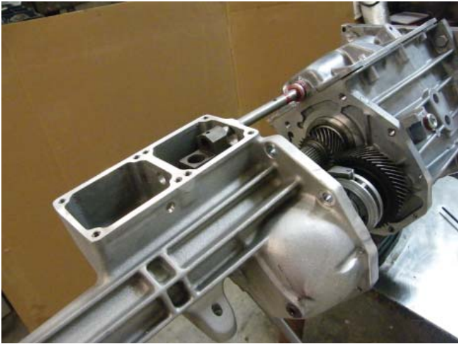
Figure 6. Here's the tailhousing just about removed from the main case assembly.
