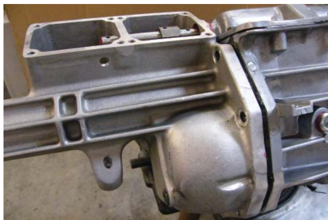
Figure 18. Here's the moment where the tailhousing rejoins the main case. I'd advise you to try this at least once and try the assembly for shift-ability before you go for a final RTV assembly. Just don't leave a split pin in a shift block. Putting one pin on top of another will really ruin your day.
